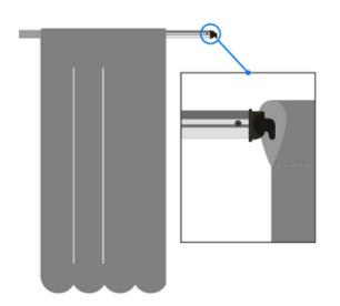
Slide the drapes over the Support bar before securing it in place.
